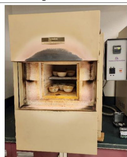
A photo of the muffle furnace. This is a high-temperature oven used to distinguish between organic and inorganic matter based on what can be burned.
