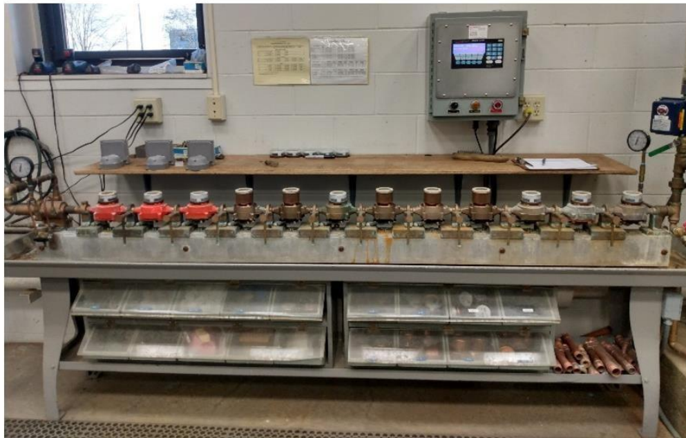
This photo shows a meter test bench in the Water Meter Laboratory full of 12 meters in the process of being tested.
